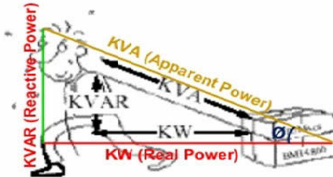
$$\text{Power Factor (pf)} = \frac{\text{kW (Real Power)}}{\text{kVA (Total Power)}} = \cos \theta$$
